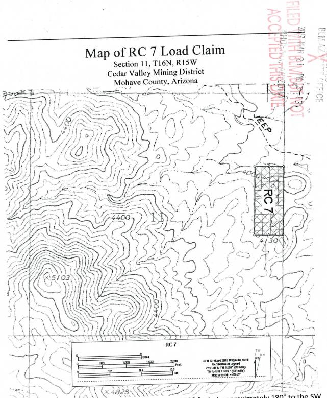
The Claim is delineated thusly: From the NW corner, 1500 feet at approximately 180° to the SW corner, then 600 feet at approximately 90° to the SE Corner, then 1500 feet at approximately 0° to the NE corner, then 600 feet at approximately 270° to the point of beginning.
