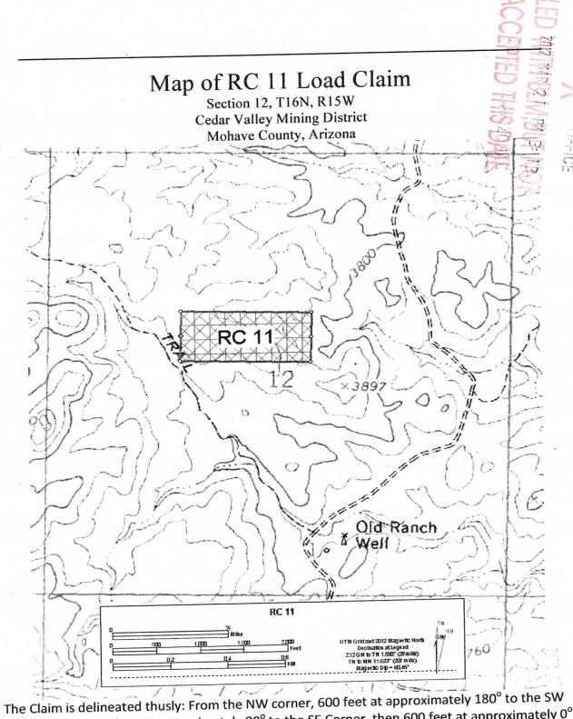
The Claim is delineated thusly: From the NW corner, 600 feet at approximately 180° to the SW corner, then 1500 feet at approximately 90° to the SE Corner, then 600 feet at approximately 0° to the NE corner, then 1500 feet at approximately 270° to the point of beginning.
