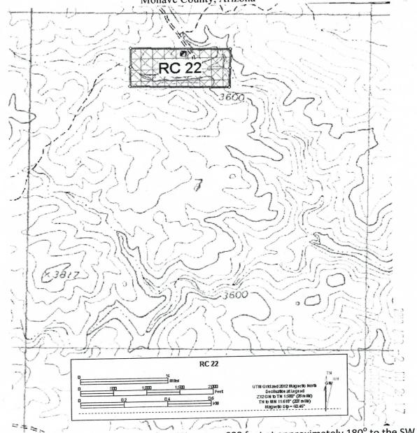
The Claim is delineated thusly: From the NW corner, 600 feet at approximately 180° to the SW corner, then 1500 feet at approximately 90° to the SE Corner, then 600 feet at approximately 0° to the NE corner, then 1500 feet at approximately 270° to the point of beginning.
