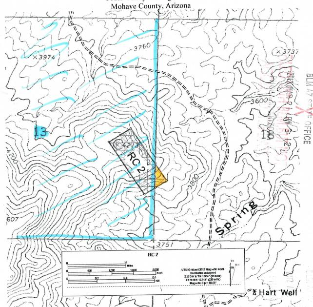
The Claim is delineated thusly: From the NW corner, 1500 feet at approximately 146° to the SW corner, then 600 feet at approximately 56° to the SE Corner, then 1500 feet at approximately 326° to the NE corner, then 600 feet at approximately 236° true North to the point of beginning.
