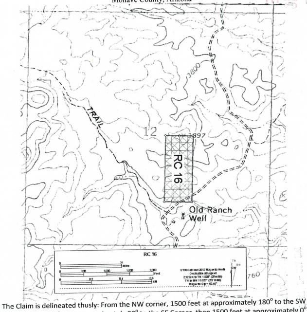
The Claim is delineated thusly: From the NW corner, 1500 feet at approximately 180° to the SW corner, then 600 feet at approximately 90° to the SE Corner, then 1500 feet at approximately 0° to the NE corner, then 600 feet at approximately 270° to the point of beginning.
