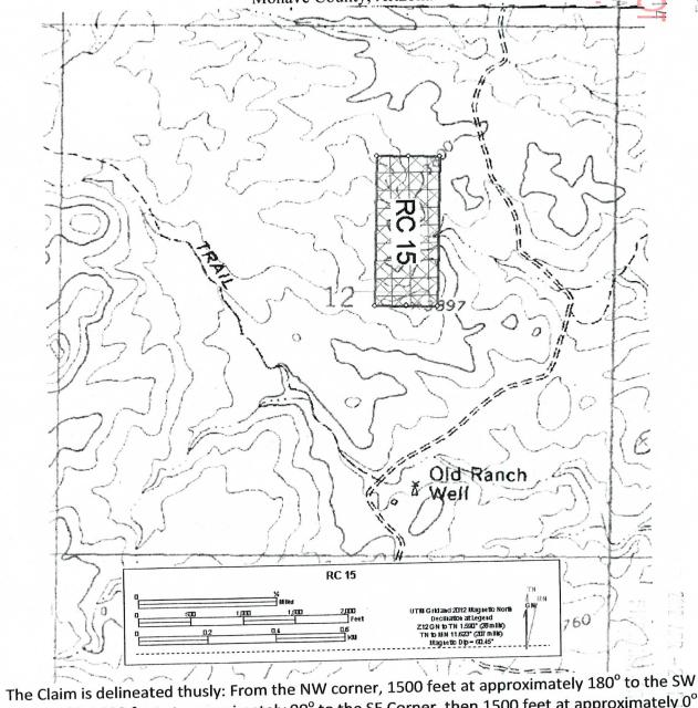
corner, then 600 feet at approximately  $90^{\circ}$  to the SE Corner, then 1500 feet at approximately  $0^{\circ}$ to the NE corner, then 600 feet at approximately 270° to the point of beginning.
